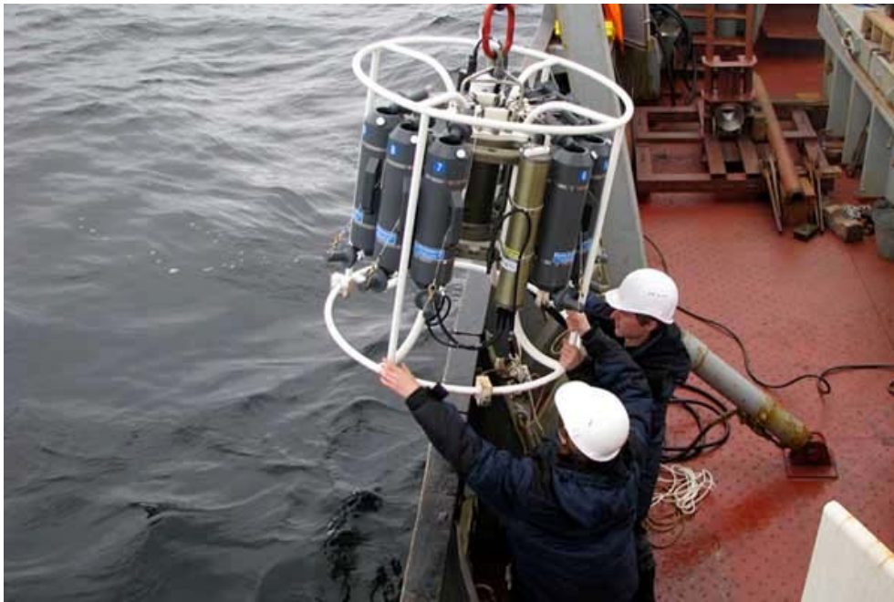
Fig. 4: Carousel water sampler (“Rosette”) Seabird 32C with attached AFM (Automatic Fire Module) and CTD (Conductivity-Temperature-Depth) Seabird 19+.
